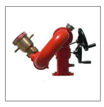
vertical and horizontal movements are controlled with handwheel driven worm gears fully enclosed and protected from the elements.
